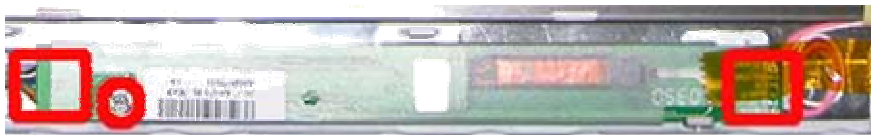
Fig. 18 Removing the Inverter Board
